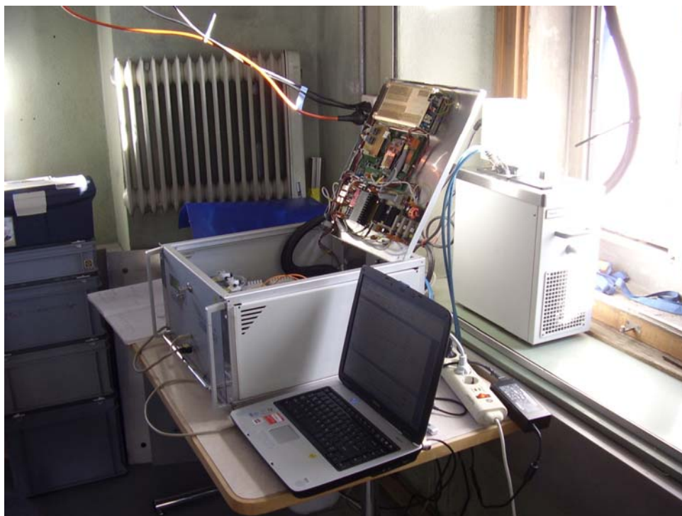
Fig. 3 LOPAP instrument in the GAW laboratory in the “Sphinx station” on the “Jungfrauoch”.
