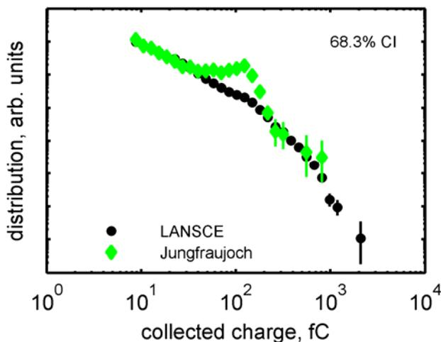
Figure 1: Differential charge collection spectra observed using ISEEM: Jungfrauoch and LANSCE compared
