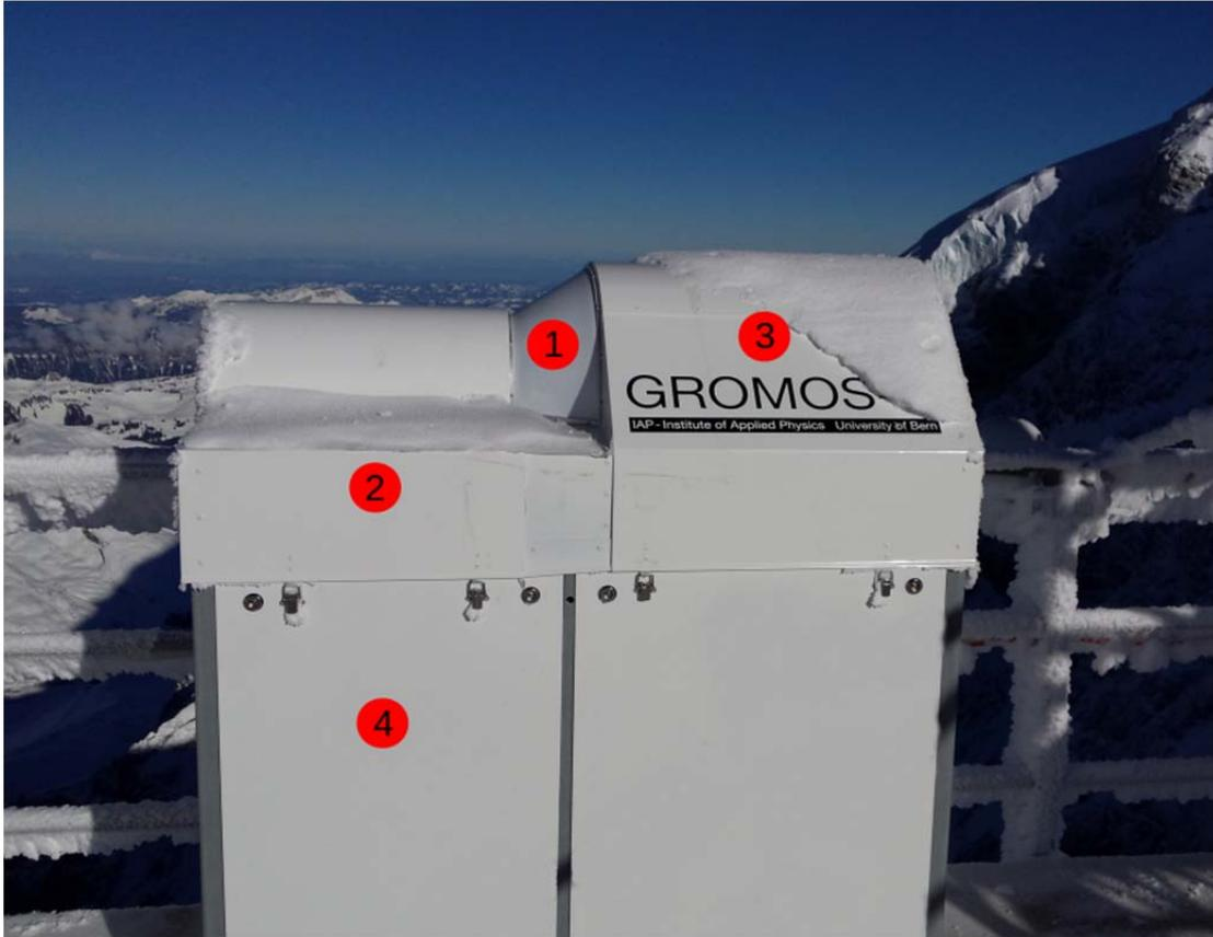
Figure 1. GROMOS-C on the Sphinx terrace during the Jungfrauoch campaign. 1: Teflon window, 2: Microwave receiver, 3: Calibration targets, 4: Computer and spectrometer.
