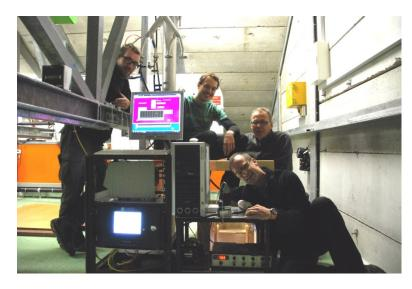
**November:** Researchers from the Paul Scherrer Institute installed an aethalometer and a condensation particle counter at the Jungfrau East Ridge station (3705 m asl, former Swisscom station), to measure aerosol microphysical properties. Similar observations have been carried out at the Jungfraujoch's Sphinx Laboratory since the 1990s. While the East Ridge site is quite close to the Sphinx, it is virtually free from local emissions.
