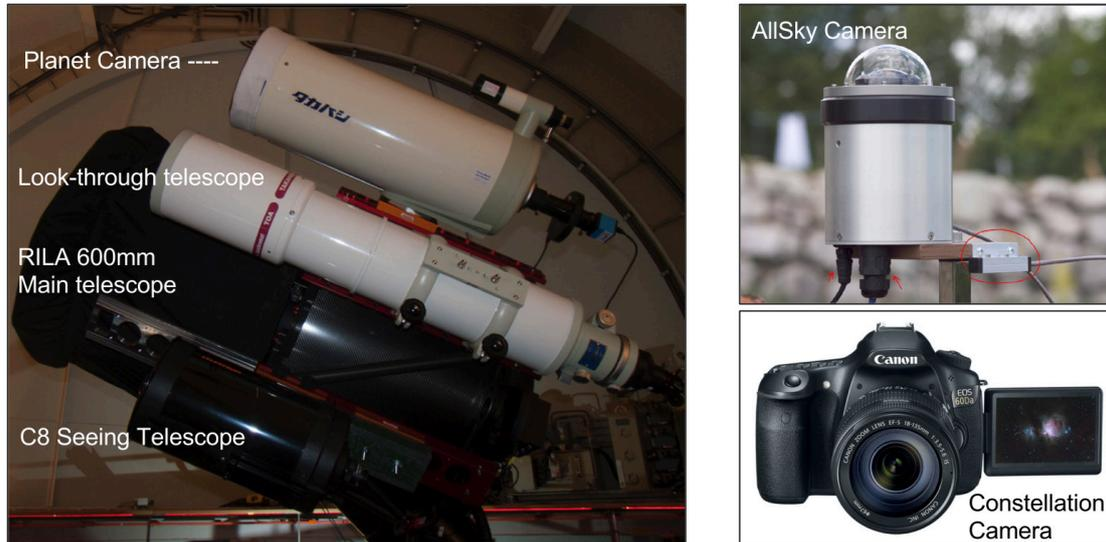
Figure 1. Available instruments at the Stellarium Gornergrat: The left panel shows the RILA main instrument (black), the Takahashi Mewlon-250 Planet Camera (blue-white), the Takahashi TAO-150 Look-Through Telescope (red-white), and the C8 Seeing Telescope. The upper right panel shows the Allsky camera and the lower right panel shows the Canon 60Da Constellation Camera.
