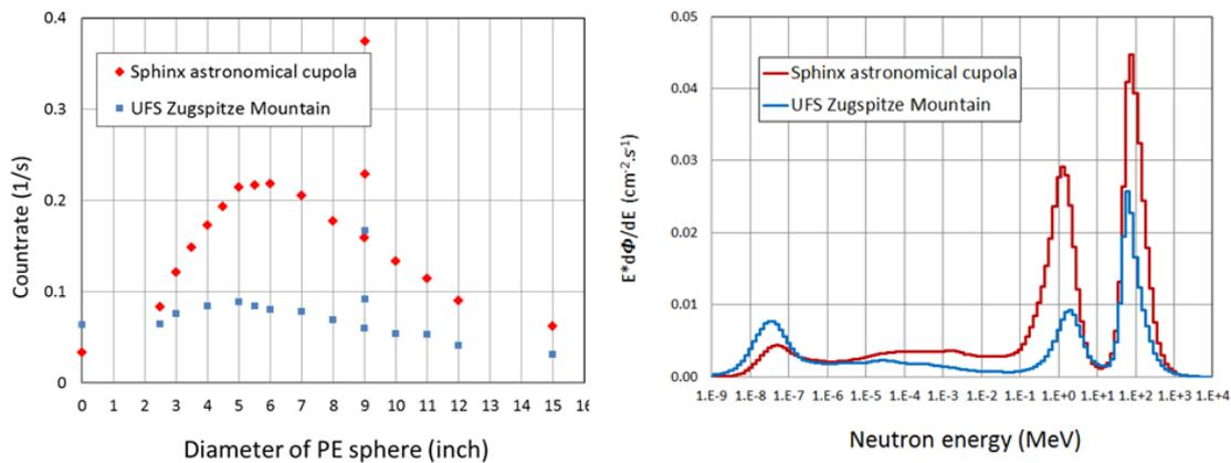
Figure 3. Mean count rates measured in June 2016 at the UFS Zugspitze and in Sphinx astronomical cupola at Jungfrauojoch (left), and resulting spectral neutron fluence rate distribution (right).
