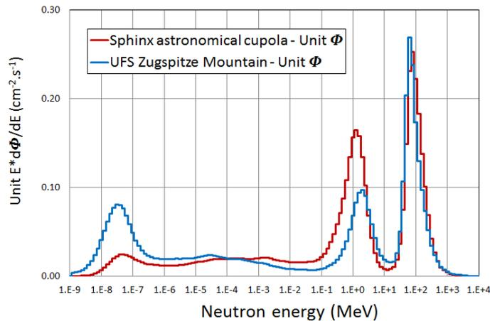
Figure 4. Comparison of spectral neutron fluence rate distribution measured in June 2016 at the UFS Zugspitze and in Sphinx astronomical cupola at Jungfrauoch (see Fig. 3 right) normalized to the total neutron fluence.
