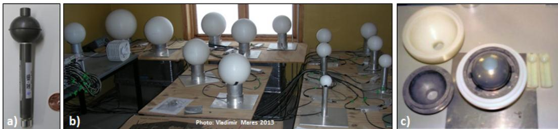
Figure 1. a) SP9  $^3\text{He}$  proportional counter (Centronic Ltd.); b) the extended range Bonner sphere spectrometer system installed at the Koldewey Station in Ny-Ålesund, Spitsbergen; c) 9 inch sphere with lead shell (Photos: V. Mares).
