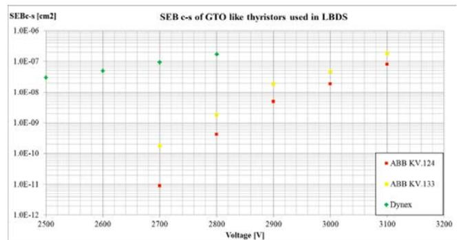
Figure 1. SEBc-s of 2 different GTO like thyristor types (both 4.5 kV rated) used in LBDS generators - Dynex and ABB made (two different production batches from ABB).
