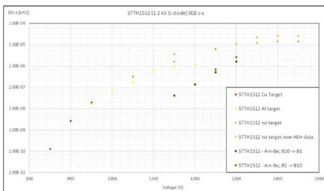
Figure 3. SEBc-s of the used HV diode (1.2 kV rated STTH1512) according to the measurements at CHARM and at Am-Be source; the later measurement is influenced by the absorption of the low energy neutrons (<12 MeV) in multiple PCBs (10) of the system under test.
