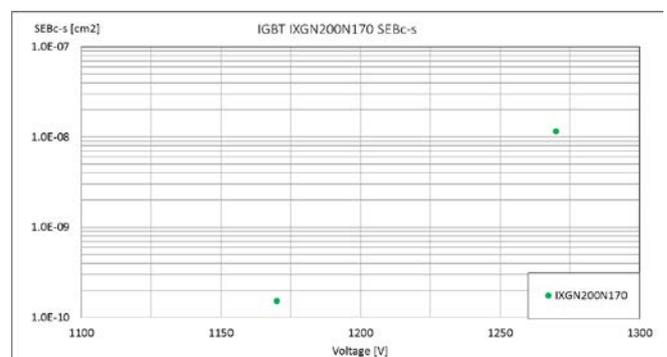
Figure 2. SEBc-s of HV IGBT IXGN200N170 (IXYS made, 1.7 kV rated) according to the measurements at CHARM.
