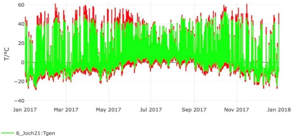
Figure 3. Time series of temperature in 2017 measured on the two PV installations at Jungfrauoch (“Joch 12” = 1993 PV installation; “Joch 21” = 2014 PV installation).
