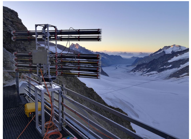
Figure 1. The primary KAPRI instrument deployed on the terrace of the Research Station, observing the Jungfraufirn area of the Aletsch glacier.
