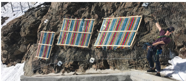
Figure 1. The frames that have been mounted underneath the research station with the different webbing samples.
