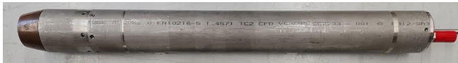
Figure 6. Acoustic equipped melting probe used for the sonar measurements (melting head on the left).
