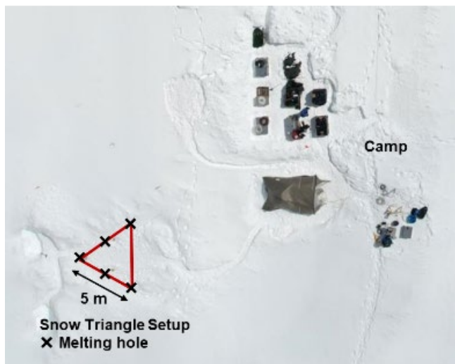
Figure 7. Birdseye view of the area probed with three acoustic melting probes.
