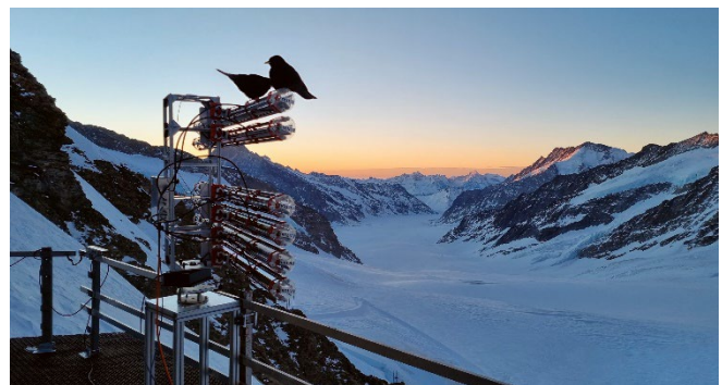
Figure 1. Primary KAPRI device observing the Jungfraufirn area from the terrace of the research station. Photo credit: Marcel Stefko.
