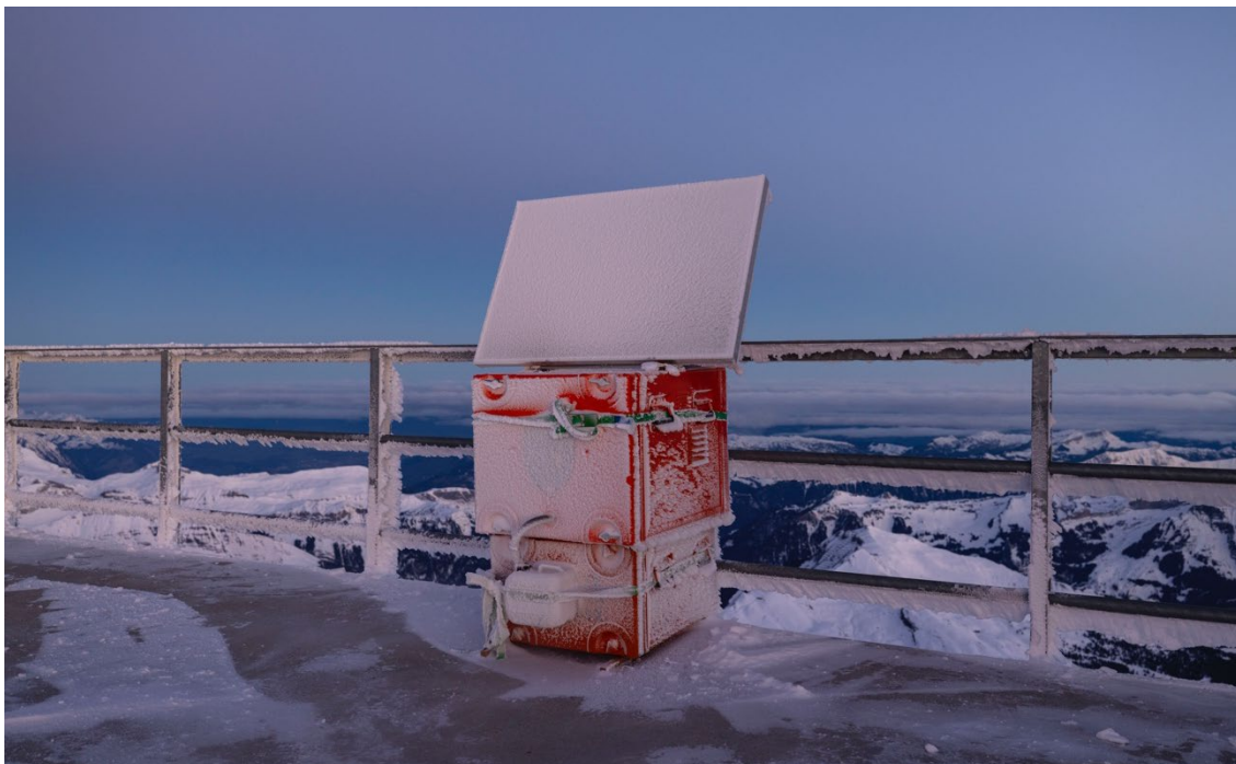
Figure 1. Methanol Fuel Cell in its weatherproof aluminium box with the attached auxiliary solar panel on the lower platform of the Sphinx observatory halfway through the February trials.
