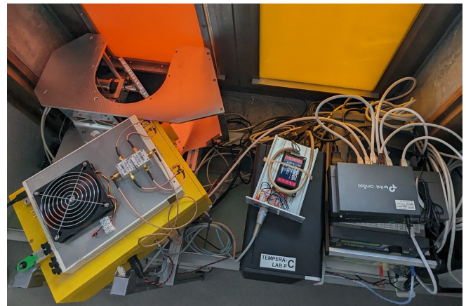
Figure 1: TEMPERA-C setup in the Sphinx-laboratory. The microwave signal is observed through the (microwave transparent) window on the left-hand side.
