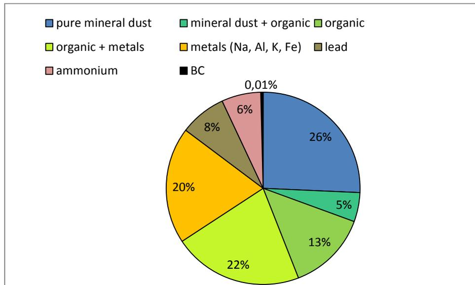
Figure 1. Relative abundance of particle types in ice residuals, measured with the single particle aerosol mass spectrometer ALABAMA using the ice counterflow virtual impactor Ice-CVI.
