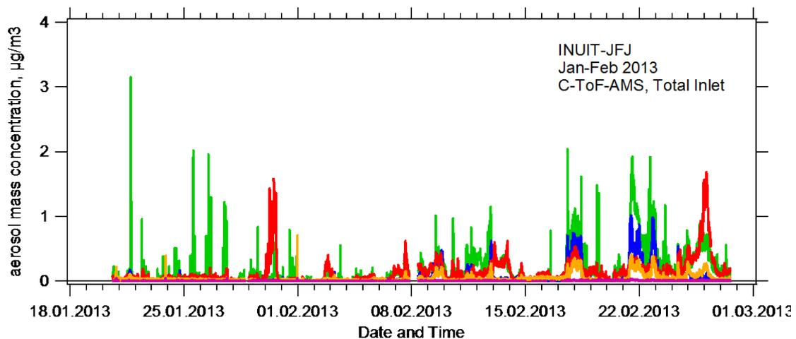
Figure 2. Total non-refractory aerosol mass concentrations (aerosol particles and ice residuals) measured using the compact time-of-flight aerosol mass spectrometer C-ToF-AMS.
