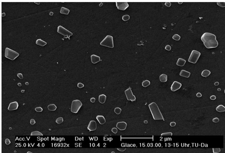
Figure 1: Secondary electron image of ammonium sulfate particles.
