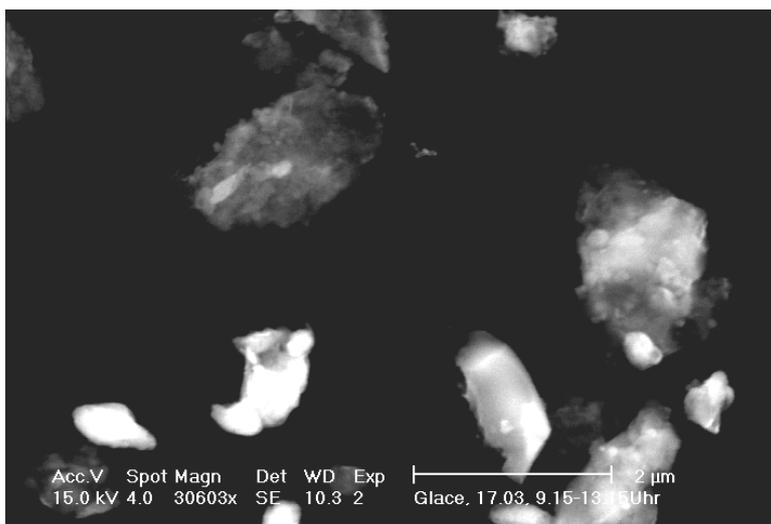
Figure 3: Secondary electron image of aluminosilicate particles.
