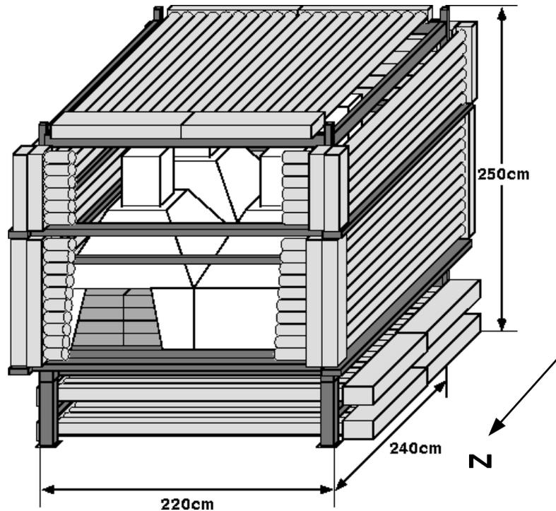
Figure 1: Configuration of the Gornergrat solar neutron detector.
