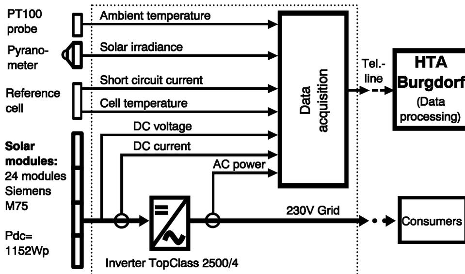
Fig. 2: Block Diagram of the grid connected PV Plant (1.152kWp nominal, 1.13kWp effective) of HTA Burgdorf at Jungfrauoch (3454m).
