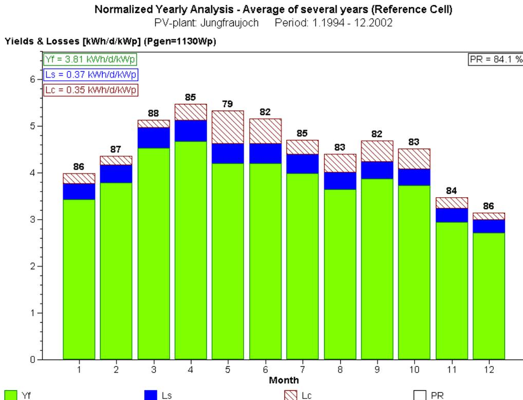
Fig. 3: Normalized monthly energy production for the average year between 1994-2002 for PV plant Jungfrauoch. Partial snow covering of the solar generator in spring causes higher  $L_c$  and lower PR values especially in the month of May and June. Production in August till October is also somewhat reduced due to the partial
