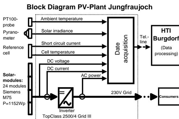
Fig. 2: Block Diagram of the grid connected PV Plant (1.152kWp nominal, 1.13kWp effective) of HTI Burgdorf at Jungfraujoch (3454m).
