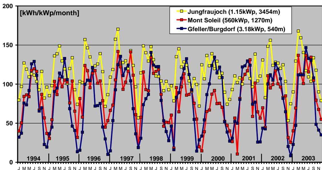
Fig. 7: Normalized monthly energy production (referred to rated PV generator power) of PV plants Jungfrauoch (1.15kWp), Mont Soleil (560kWp) and Gfeller/Burgdorf (3.18kWp) in the years 1994 to 2003.
