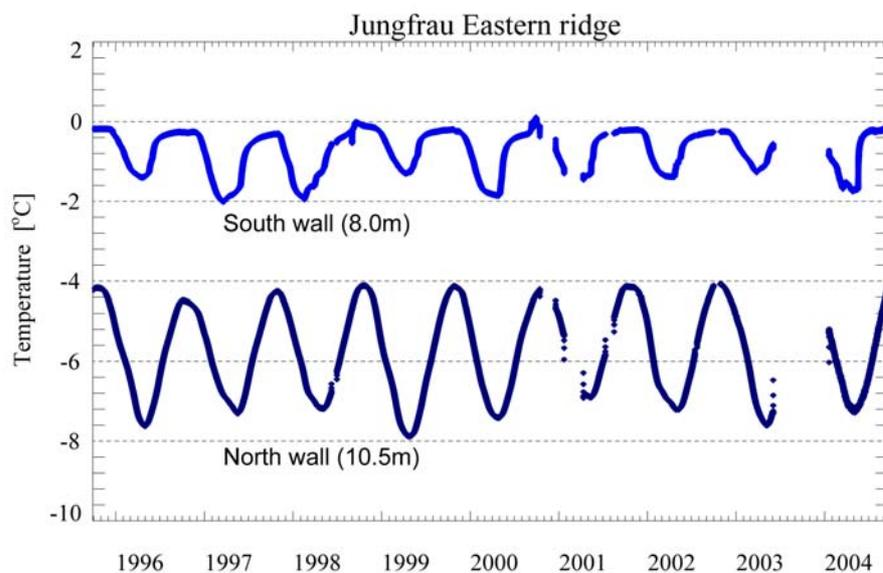
Temperature variations of ca. 10m-depth (from the surface of rock wall) thermistors are shown in the figure. It has a distinct difference in temperature between north and south. North wall has the lower value of temperature and the larger amplitude of
