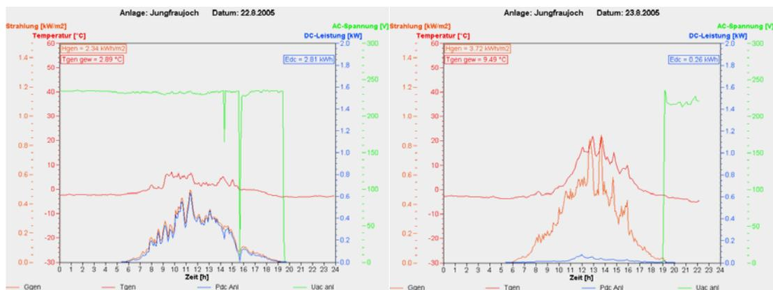
**Figure 6:** The AC power outage (green curve) during the flooding period of August 22<sup>nd</sup>/23<sup>rd</sup>, 2005 as recorded by the photovoltaic power plant operated in the High Altitude Research Station Jungfrauoch by the Berner Fachhochschule, Hochschule für Technik und Informatik, Burgdorf (courtesy Prof. Heinrich Häberlin).
