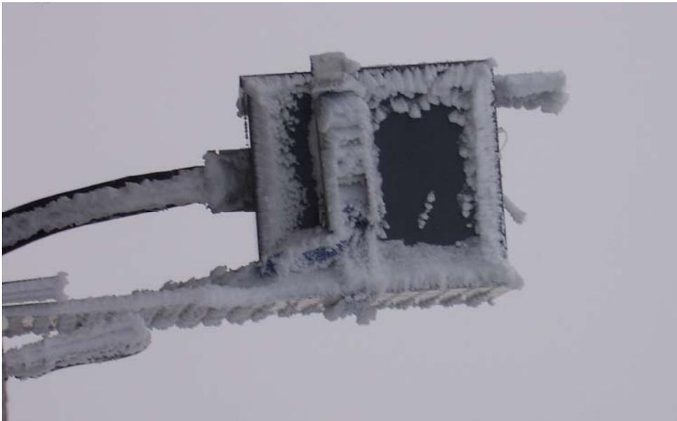
Fig. 4 External sampling unit of the LOPAP instrument during strong frost formation caused by a super saturated cloud event on the 04.-05. November 2005.
