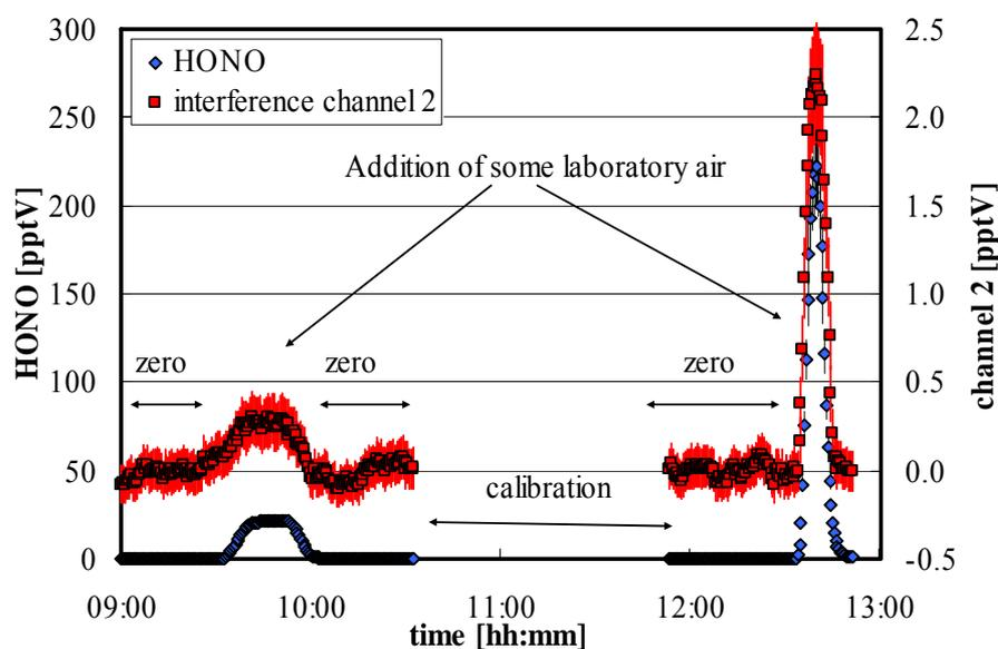
Fig. 1 Sensitivity and time response tests of the optimized LOPAP instrument. The instrument was running under zero air. HONO was added by decreasing the flow rate of the zero air slightly below the flow rate of the instrument, thus measuring very diluted laboratory air. To demonstrate the sensitivity of the instrument the signal from the interference channel 2 is also shown.
