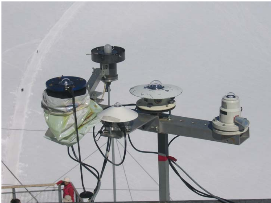
Figure 2: Further radiation detectors: on the left input optics of the spectroradiometer for global irradiance (dark blue) and actinic flux density (black) All input optics of the spectroradiometer are connected with quartz fibres (6 m) to the spectroradiometer itself, which is installed in the laboratory just below the terrace. The 3 white detectors are broadband instruments for global, UVA and UVB irradiance.
