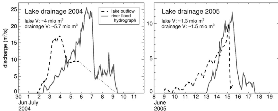
Fig. 2 Outflow from Gornersee and corresponding discharge record (in which the contribution of the glacier melt was subtracted) in the Gornera river at Grande-Dixence gauging station near the glacier snout for the years 2004 and 2005. Note that after July 5 2004, no lake level records were available.
