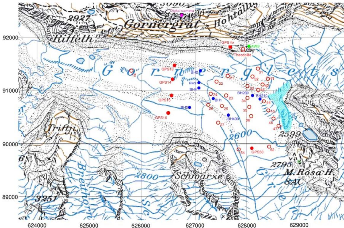
*Fig. 1 Map of the study site (2005). The locations of the theodolite survey stakes, GPS-stations and boreholes are indicated by the open red circles, solid red circles, and solid blue circles, respectively. The seismicity was measured in the hatched red-areas (left 2005 and right 2004) and Gornersee is shown in light blue.*
