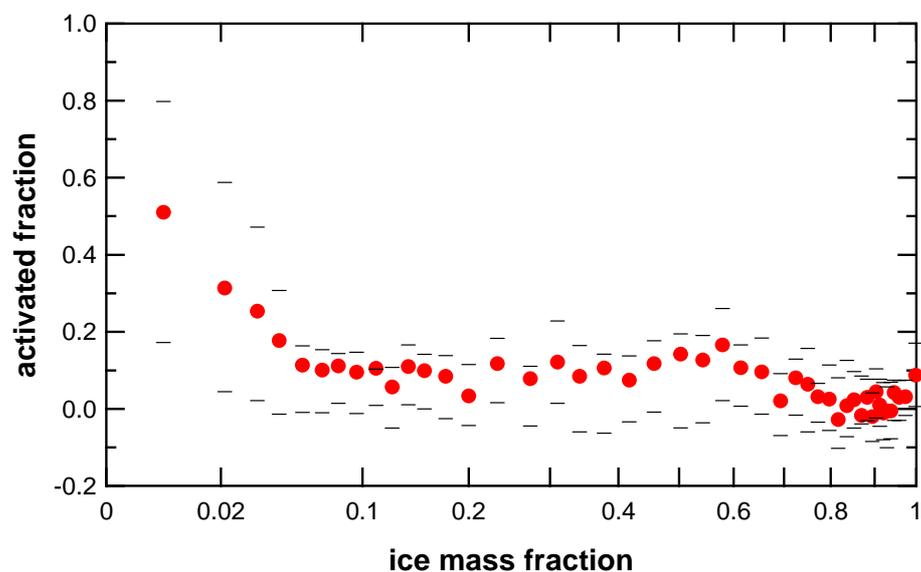
Figure 2. Activated fraction of particles as a function of ice mass fraction in the cloud. Circles denote the average, while horizontal stripes denote the 25 and 75 percentile values.
