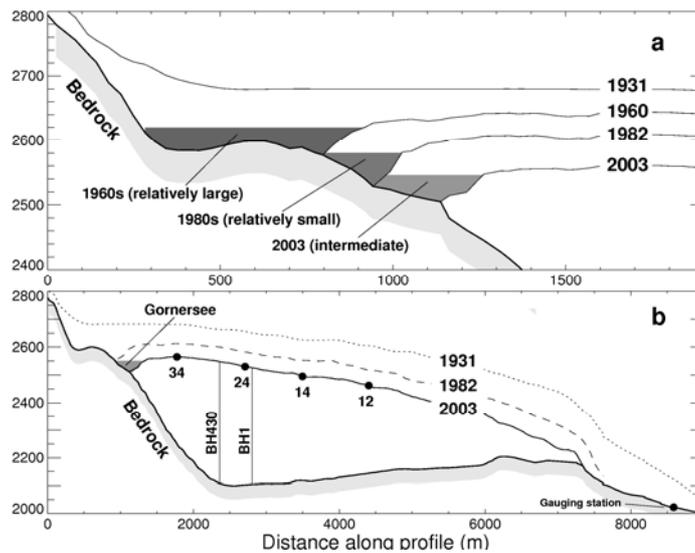
**Fig. 2:** (a) Schematic profile of the *Gornerssee* evolution during the past decades. (b) Longitudinal profile of the *Gornergletscher* tongue. Bed topography was obtained from radio-echo soundings. Two boreholes and four stake locations are indicated.
