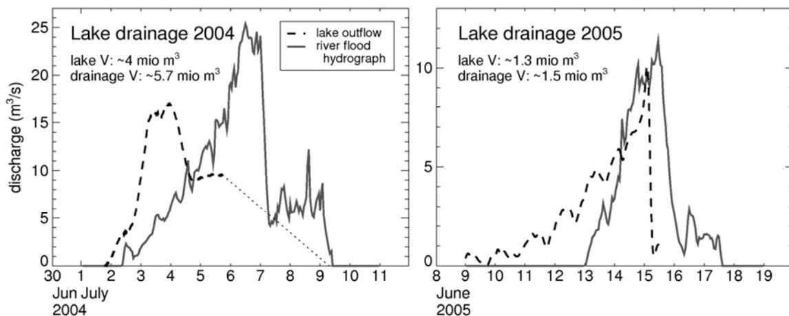
**Fig. 6:** Outburst from *Gornersee* and corresponding discharge record (in which the glacier melt contribution was subtracted) at the *Gornera* River at *Grande Dixence* gauging station near the glacier snout for the years 2004 and 2005. Note that after July 5 2004, no lake level records were available.
