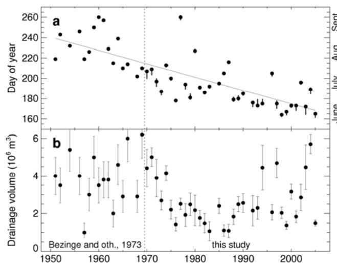
**Fig. 4:** (a) Evolution of lake outburst timing. (•) correspond to the dates of peak discharge. Vertical bars show the duration of the drainage events. (b) Time series of drainage volumes with corresponding error bars.
