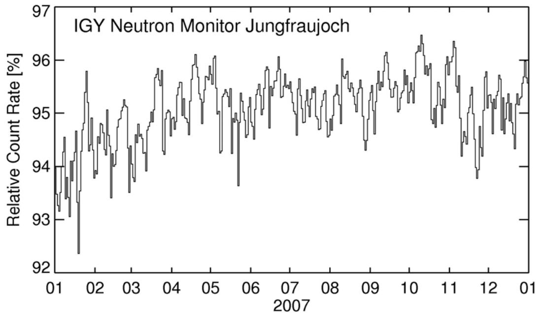
Figure 1: Relative pressure corrected daily counting rates of the IGY neutron monitor at Jungfrauojoch for 2007.
