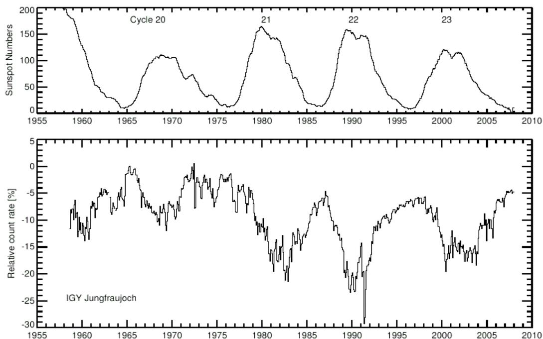
Figure 2: Smoothed sunspot numbers (top panel), pressure corrected monthly average counting rates of IGY neutron monitor at Jungfrauojoch (bottom panel) for the years 1958-2007. The neutron monitor count rate is expressed in relative units with respect to May 1965.
