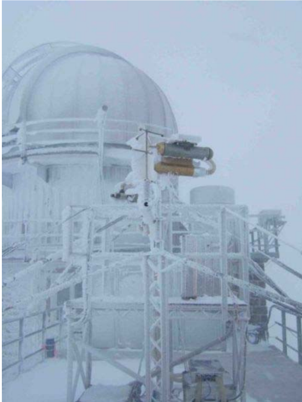
March: CLACE 6 (CLoud and Aerosol Characterization Experiment) at Jungfrau-joch. Cloud Particle Imager (CPI) and Forward Scattering Spectrometer Probe (FSSP) firmly installed on the Sphinx platform to withstand a snowstorm.
