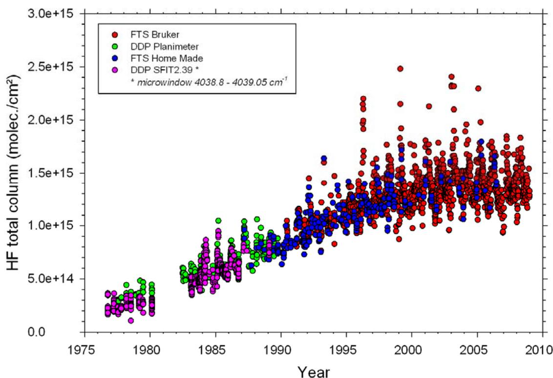
Figure 2 – Total column of fluorhydric acid HF above Jungfraujoch, derived from spectra acquired by 3 different instruments: the 7-m grating spectrometer from 1976 to 1989 (“DDP”), the home-made Fourier transform spectrometer (FTS) from 1985 to 2006, and the Bruker FTS from 1990 to now. Grating spectra have been analysed by two different methods: in the 80s with a planimeter instrument (green dots), and recently with the SFIT2 software (pink dots).
