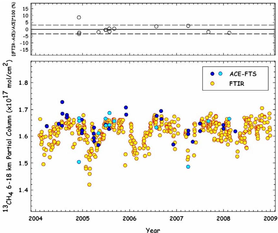
Figure 1 - Daily mean  $^{13}\text{CH}_4$  6-18 km partial columns time series as observed by the ACE-FTS space instrument (blue and light blue circles) and by FTIR spectrometry at Jungfraujoch (yellow circles). Light blue circles correspond to coincident days between satellite and ground-based data. Top panel reproduces relative differences between FTIR and ACE-FTS data (solid line: mean relative difference; dotted lines:  $1-\sigma$  standard deviation on the mean).
