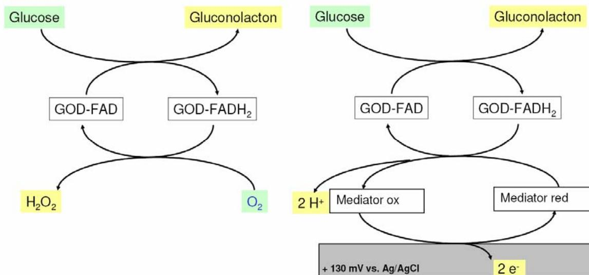
**Figure 1: Amperometric glucose detection using glucose oxidase (GOD) as enzyme. Left: Natural regeneration of GOD by oxygen. Right: Regeneration of GOD using a mediator.**
