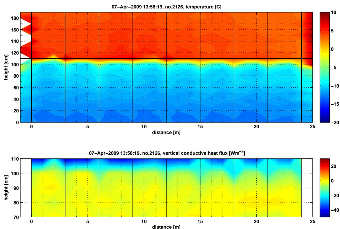
Figure: Temperature transect and corresponding vertical conductive heat flux near the snow surface.
