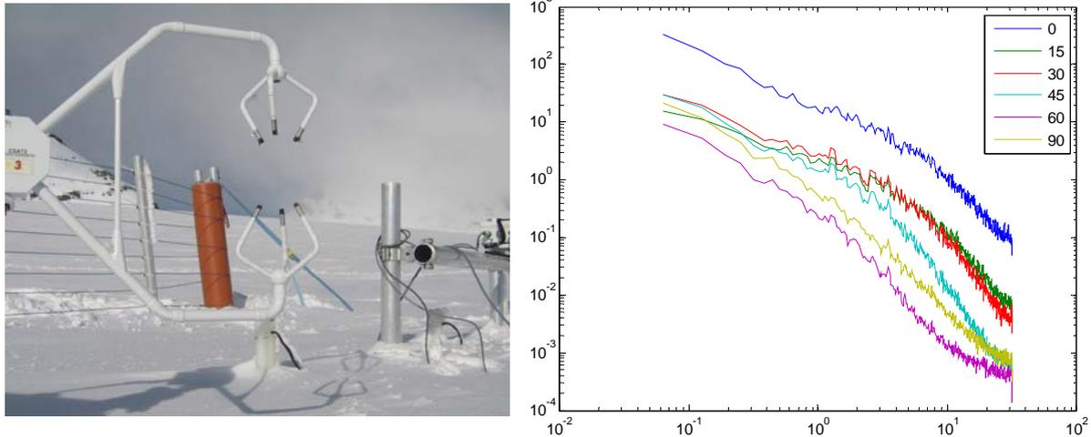
Figure: Setup of pressure poles and sonic anemometer. Example of power spectra at different depths.
