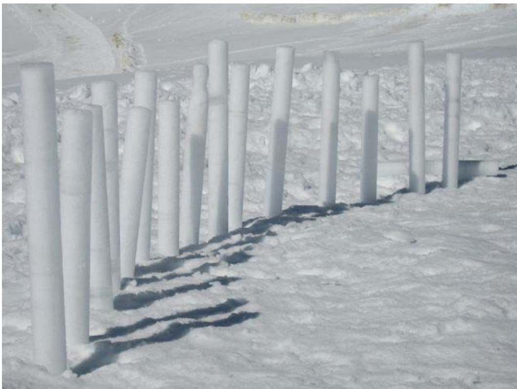
October: Fence of firn cores recovered during a test drilling campaign on Jungfrauojoch (team: FS INVENTOR SA, University of Maine and Paul Scherrer Institut).
