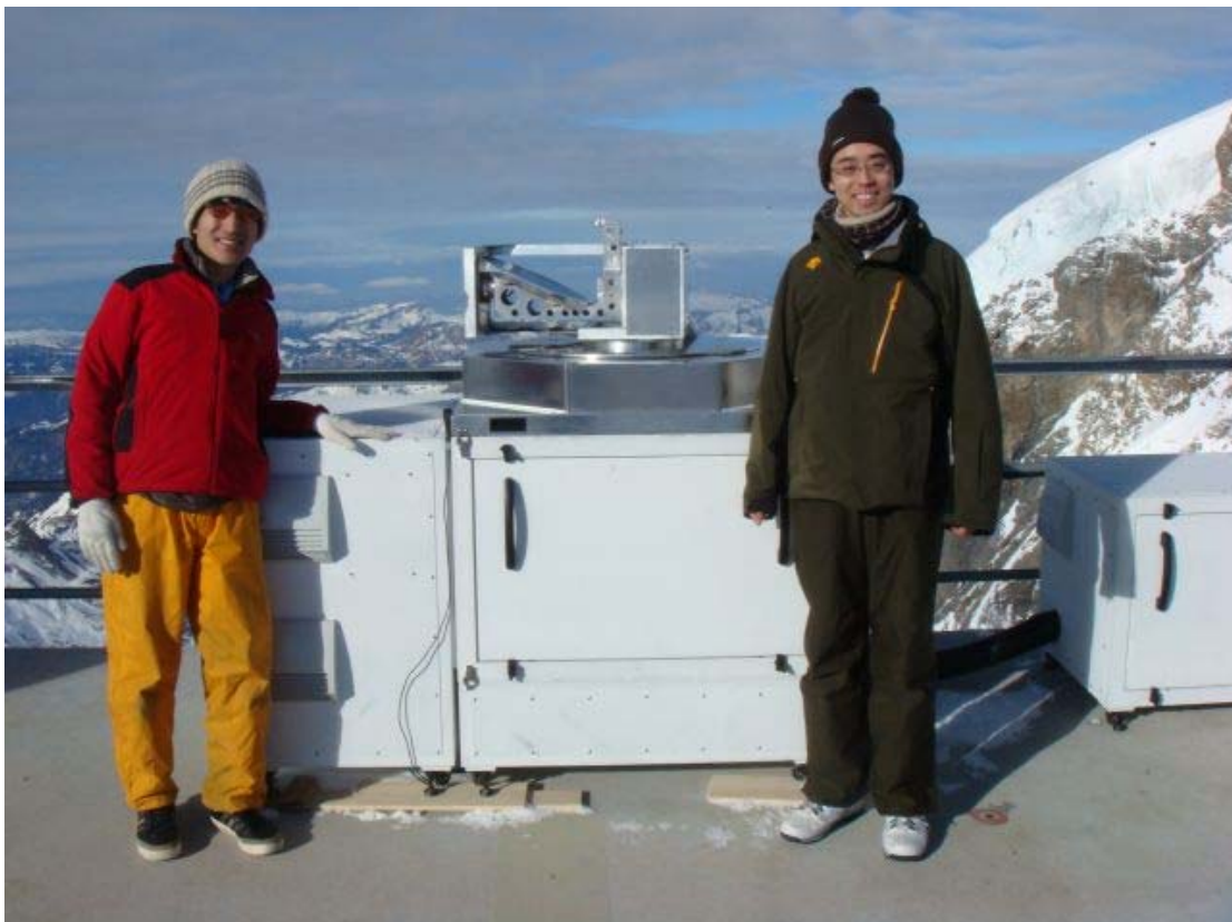
February: The University of Tsukuba, Japan, is testing its 30cm radio telescope at the Research Station Jungfrauoch by mapping the Milky Way in CO and Cl lines. The telescope is equipped with a 4-K cooled 500 GHz sensitive detector. The final destination of the telescope will be the Antarctic.
