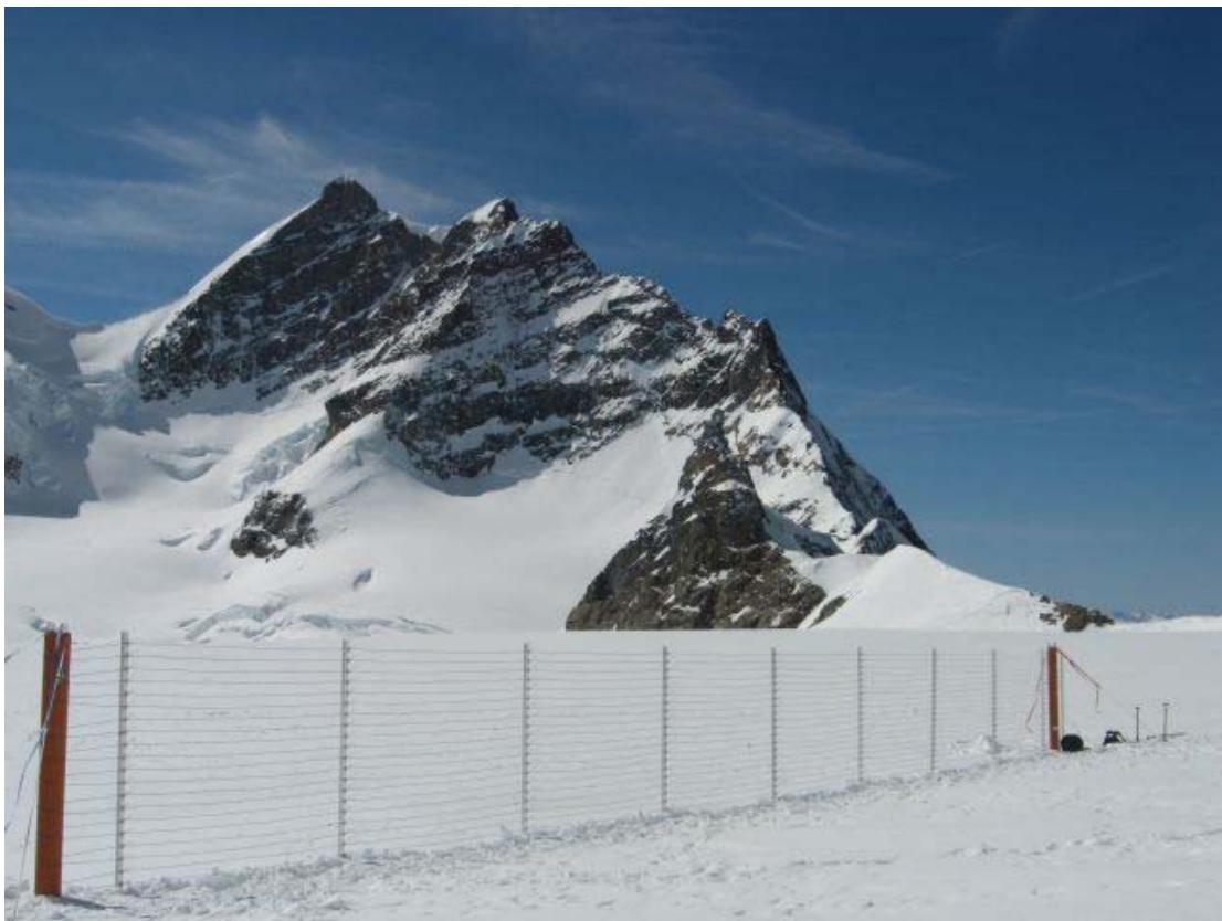
April: Snow atmosphere interaction experiment: EPFL-EFLUM deployed a 25m long and 2m tall 'fence' consisting of a fiber optical cable to measure a temperature transect in the snow pack with high spatial resolution. Measurements are based on a Raman-optical TDR system. (Photo courtesy of Hendrik Huwald, École Polytechnique Fédérale de Lausanne)
