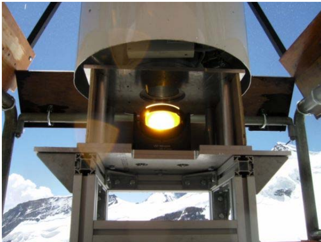
July: The solar tracker installed by the UK's National Physical Laboratory that is interfaced with a high resolution FTIR for measuring the radiative transfer through the atmosphere as part of the UK's CAVIAR project on the water vapour continuum. ( http://www.met.reading.ac.uk/caviar/ )
