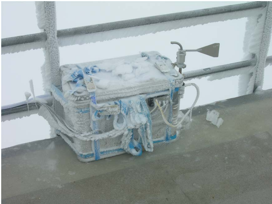
HOLIMO during CLACE 2010 on the Jungfraujoch. The bent tube with the vane is the inlet that moves to the direction of the wind automatically
