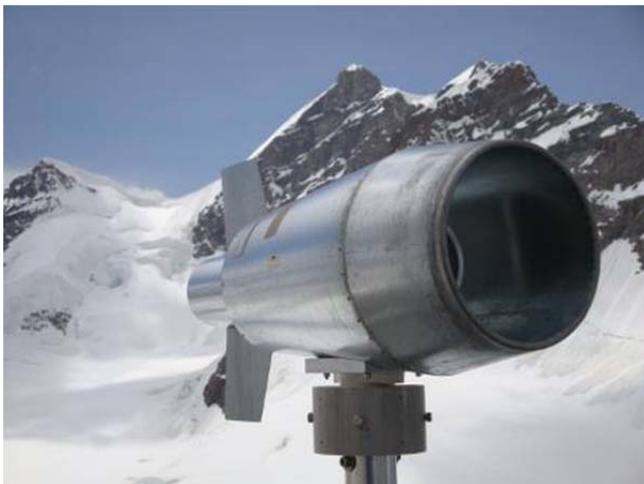
***Figure 1.** Picture of the original flow through air sampler installed at Jungfraujoch (picture Matthew MacLeod, Stockholm University).*
