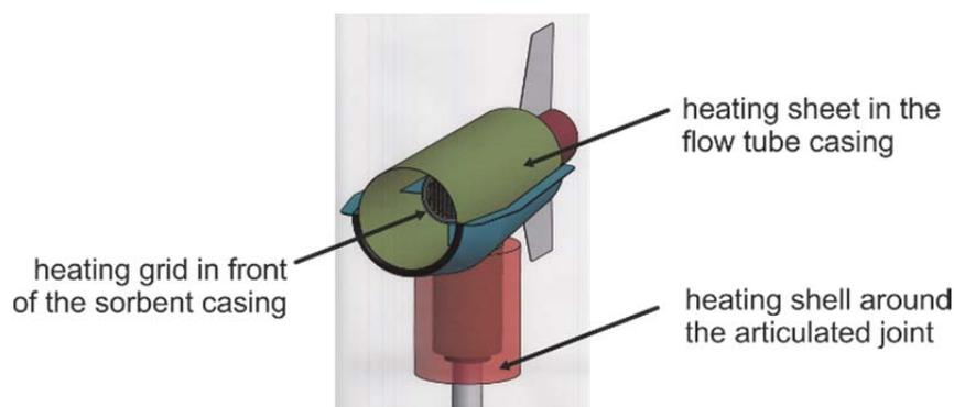
**Figure 2.** Sketch of the newly constructed flow through air sampler.
