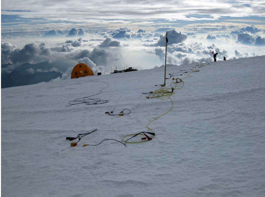
Photo 1: Deployment of the geophone line along a profile marked with bamboo poles towards East. The camp is in the background. Photo: Anja Diez, AWI
