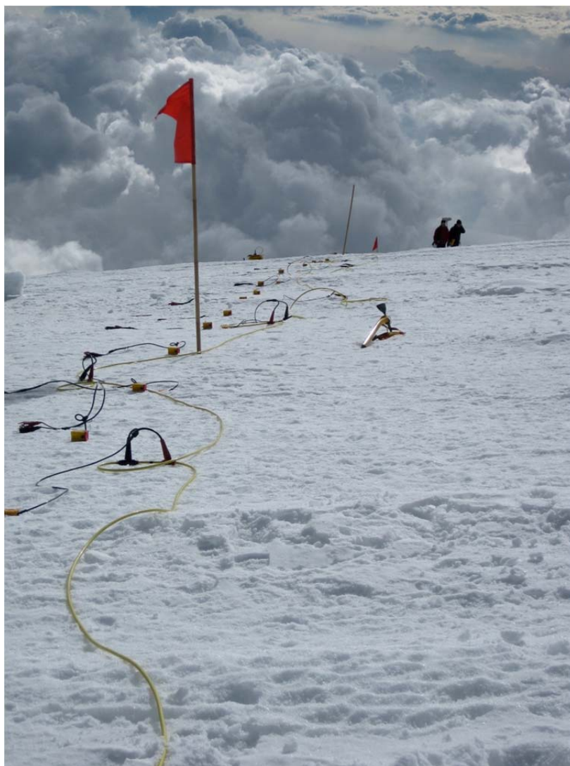
Photo 2: Deployment of the geophone line along a profile marked with bamboo poles towards East, Lago Maggiore is in the background. Photo: Anja Diez, AWI
