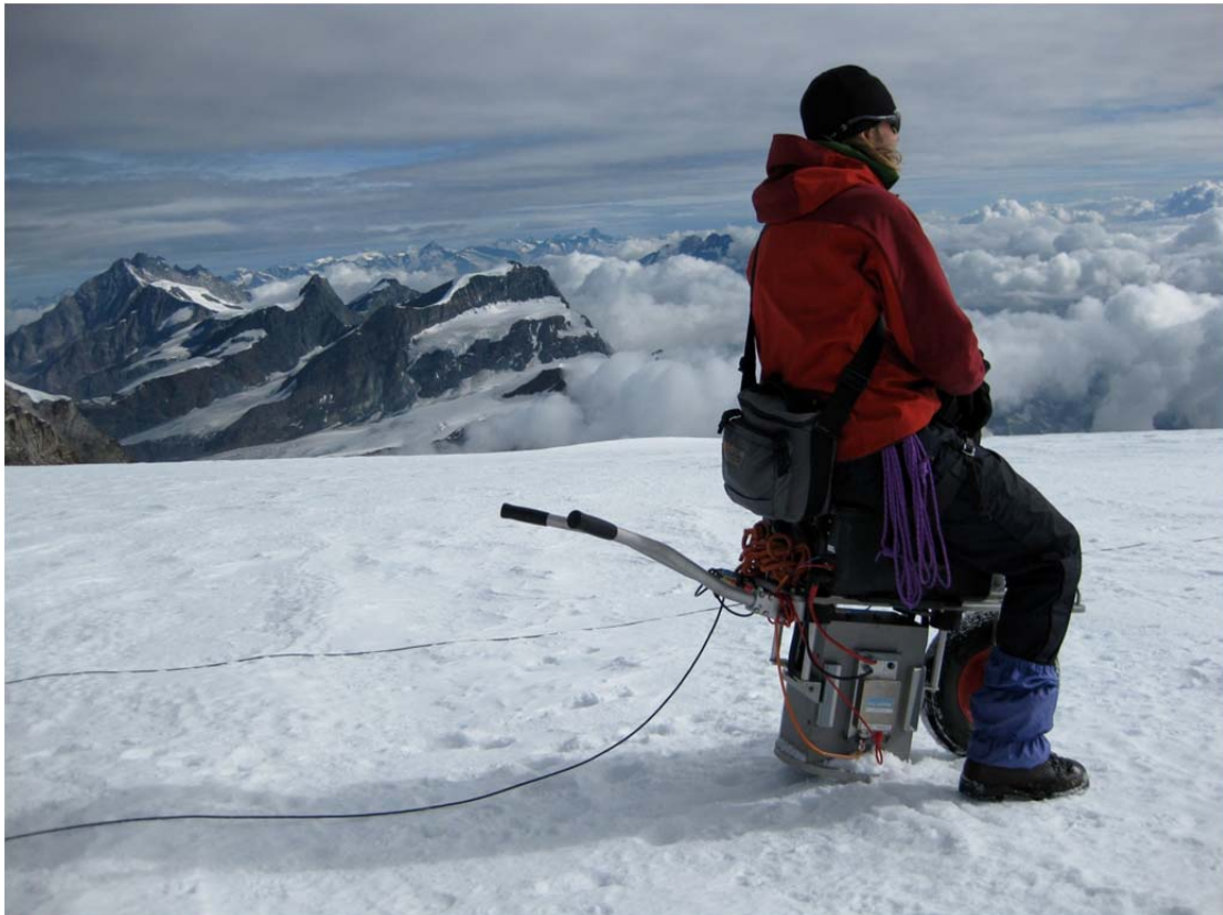
Photo 3: The EIViS vibroseis source with additional weight on top to increase pressure at the base. Photo: Anja Diez, AWI
