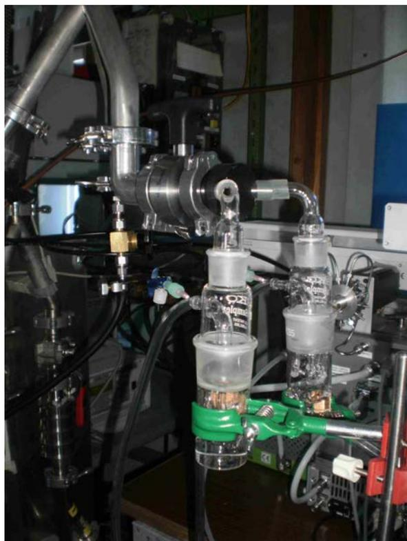
**Figure 1.** Liquid impingers connected to the total aerosol inlet provided by the Laboratory of Atmospheric Chemistry of the Paul Scherrer Institute (PSI) at the Sphinx laboratory, High Altitude Research Station Jungfraujoch, August 2011.
