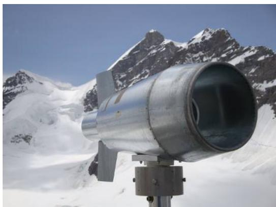
**Figure 1.** Picture of the original flow through air sampler installed at Jungfrauoch (picture Matthew MacLeod, Stockholm University).
