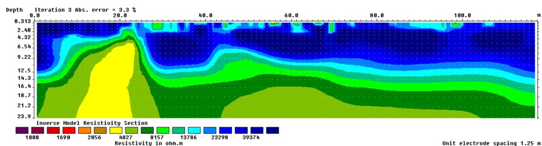
**Figure 1.** ERT inversion model along the Stockhorn plateau (W to E) showing specific electrical resistivity in a 2-dimensional cross-section. High resistivity values (blue) correspond to higher ice contents within a more-weathered surface layer, reduced resistivities (green/yellow) correspond to low-porosity but still frozen bedrock below.
