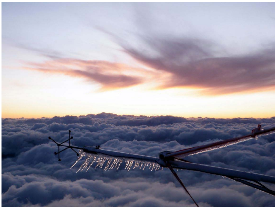
July: A Sonic Anemometer (provided by the University of Basel) in front of a nice summer sunset. This measurement is being conducted within a campaign (CLACE) where the interaction of aerosol particles with cloud droplets is being investigated.
