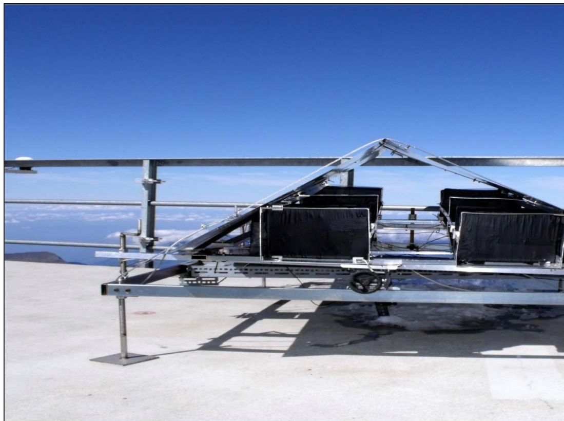
Figure 1: Detector located at the Sphinx. The four black boxes contain the tiles, SiPM and amplifier. They are 60 cm apart and 160 cm along the path of flight of horizontal tracks.
