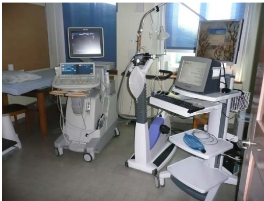
Fig. 1: Technical equipment at the Jungfrauoch: from left to right: echocardiography equipment, ergometer with set-up for inert gas rebreathing measurement (balloon mounted to the mouth piece) and cart with gas analyser (Innocor ® ) and monitor.
