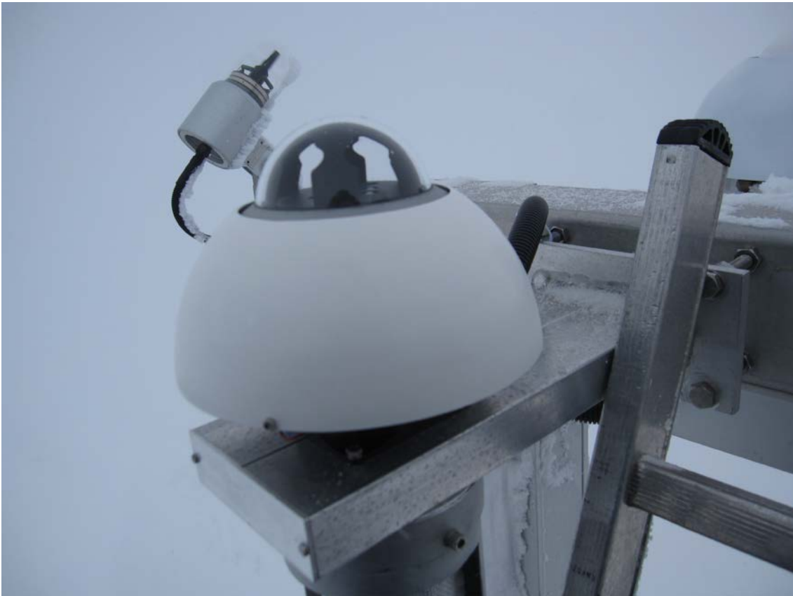
Figure 1: New instrument (SPN1 by DeltaT) installed on the radiation bridge.
