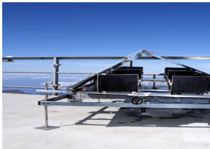
Figure 1. Prototype detector installed at the Sphinx (HFSJG) to test upward/downward particles' separation and environmental effects.
