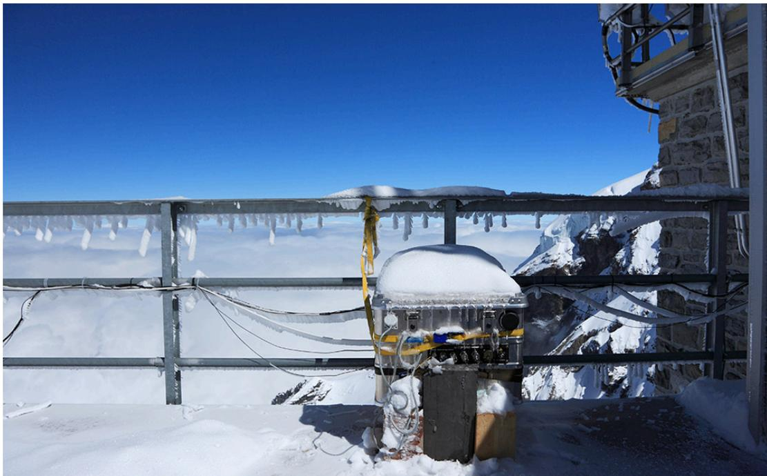
*Figure 1. Methanol Fuel Cell in its weatherproof aluminium box on the lower platform of the Sphinx observatory during the spring trials.*
