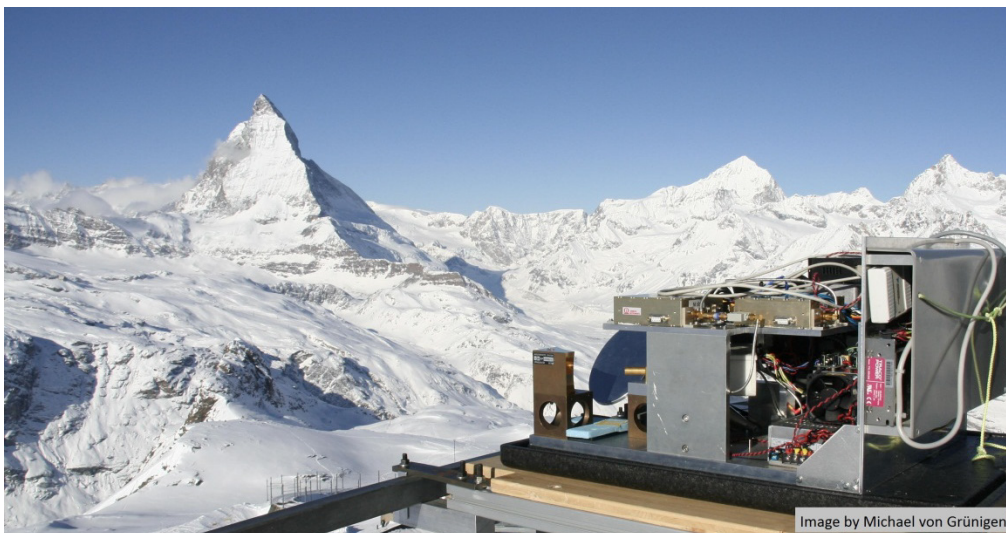
Figure 1. 340 GHz radiometer breadboard with the STEAMR receiver prototype, calibration optics and thermal stabilization installed outdoors at the Gornergrat Observatory (instrument housing removed).
