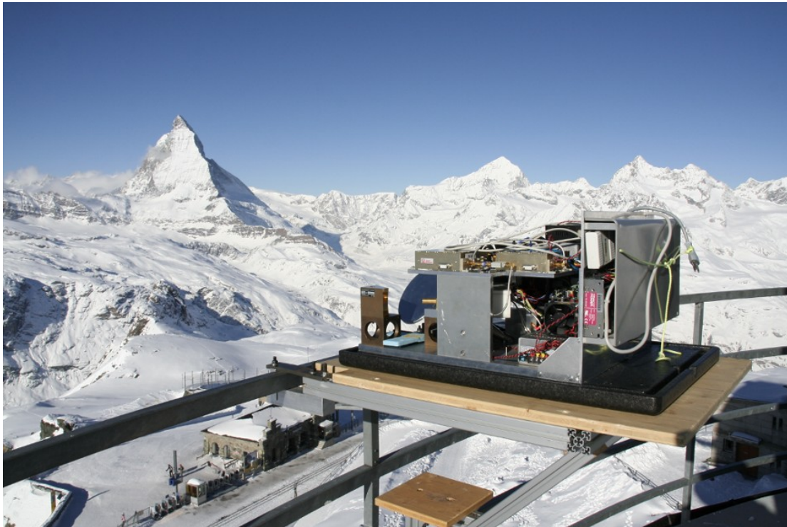
March: A project of the Institute of Applied Physics, University of Bern: Atmospheric remote sensing with a STEAMR (Stratosphere-Troposphere Exchange and Climate Monitor Radiometer) 340 GHz receiver prototype at Gornergrat.
