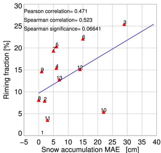
Figure 2. Relation between radar-retrieved fraction of rimed snow with respect to snow accumulation. Overall snow accumulation is higher when snowflakes are rimed.
