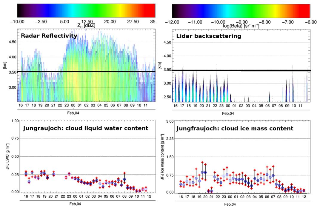
Figure 1. Complementarity of radar observations and lidar observations (both instruments pointing vertically), and in-situ (Jungfraujoch) cloud measurements. The altitude of the Jungfraujoch measurement site is indicated by a black line on the radar and lidar time-height plots.
