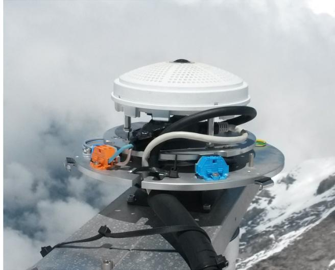
Figure 1. Hemispherical Cloud Camera of type MOBOTIX mounted on the radiation platform of Meteoswiss on the Sphinx terrace at Jungfraujoch. The weather protection dome has been removed on this picture (picture courtesy Ch. Aebi, June 2014).
