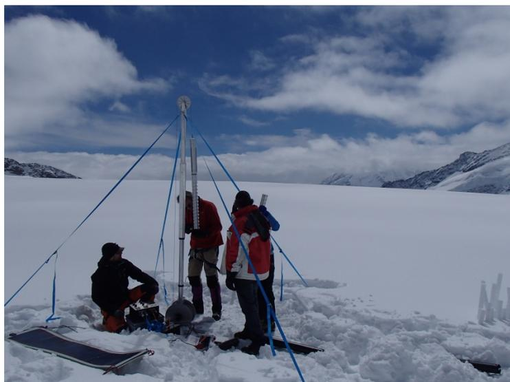
Figure 1. Test of the shallow firn drill FELICS small equipped with a light-weight winch at the Jungfraufirn.
