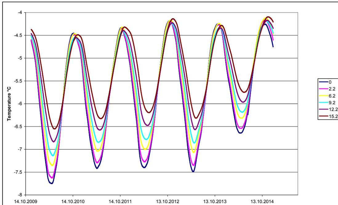
Figure 1. Borehole temperatures in the Jungfrau Ostgrat N borehole (Legend: 0 is located 6 m from the outer surface of the rockwall).
